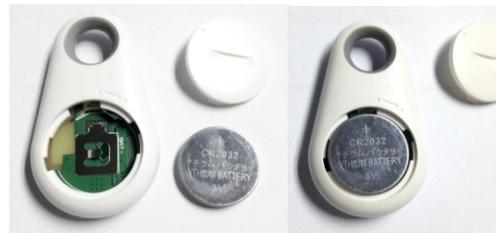
Step 2. Press and fit the cell on below position, Negative pole towards the down side.
