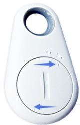
Step 3. Put back the bottom cover, clockwise rotation to close.
